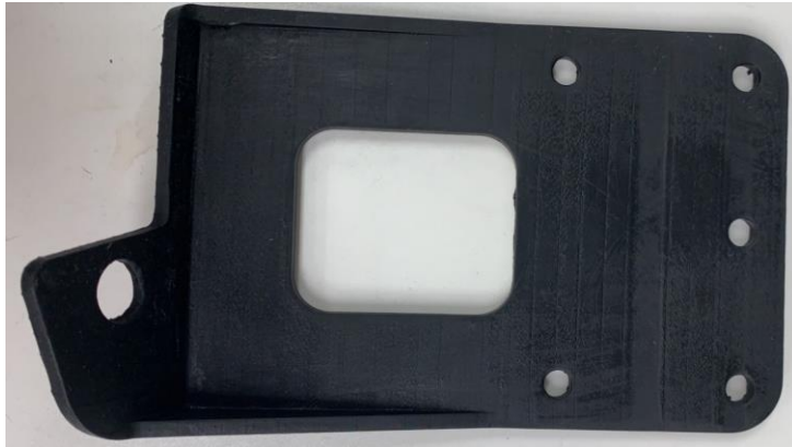
One successfully printed camera mount.
