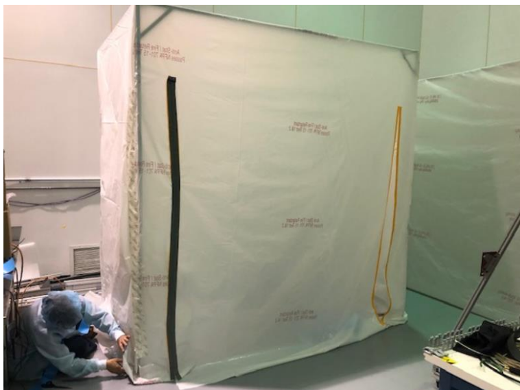
Mindy Leffel attaching non-flammable plastic sheet to aluminum frame.
