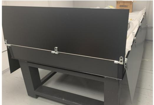
Side walls on optical table in EEL 108 sub-room. The walls on the 10-ft sides are in the down position. The wall in the closest 5-ft side is in the installed position and is held in place by magnetic holders.
