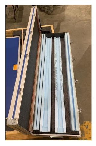
Photo showing three sets of padding for bars inside of a quartz bar case. Middle set is opened to show both halves of padding and cutouts for bars. The other two sets are on their sides.
