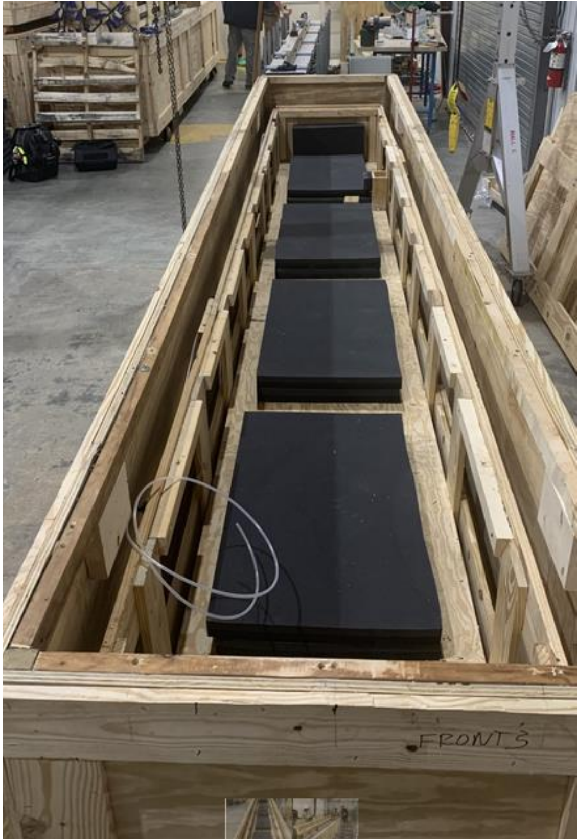
Photo of interior of one modified crate showing foam supports and air-suspension tubing.
