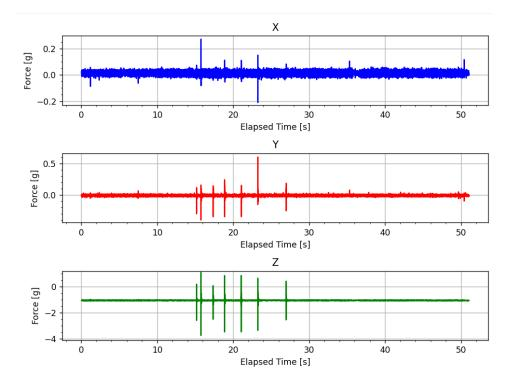
Screenshot of accelerometer's *x*-, *y*-, and *z*-axis measurements during benchtop test. Spikes in plots are from bumping table near accelerometer.
