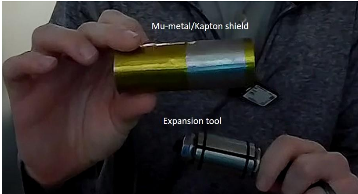
Figure 2. An expansion tool is used on the mu-metal/Kapton shielding tube to increase the inner diameter so that it will fit on the light-guide and PMT
