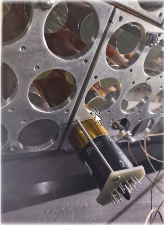
Figure 1 shows a single PMT installed on one of the lightguides of a supermodule.
