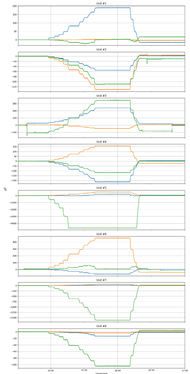
FIG. 2. X (blue), Y (orange), and Z (green) components of each of the field mapping units.
