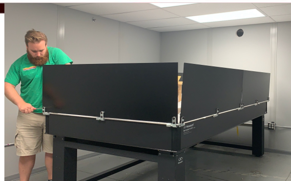
Interior of EIC DIRC's laser controlled area in EEL 108. Optical table (5'X10' with 1.5' sidewalls) is for the laser, optics, and motorized stages.
