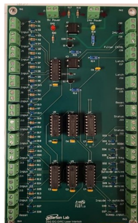
Fabricated laser interlock PCB
