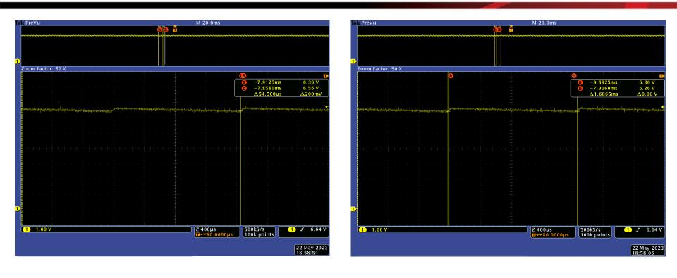
6% supply output measures 200 mV peak to peak, with a period of 593 Hz
