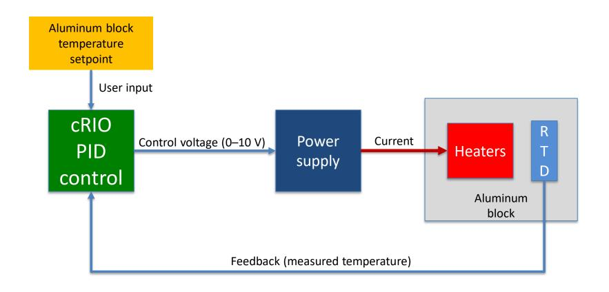
The controls software receives the aluminum block temperature setpoint from the user input and the actual temperature of the aluminum block as feedback. It provides an analog signal to the power supply (0–10 V) and proportionally controls the output of the supply in percentage.
