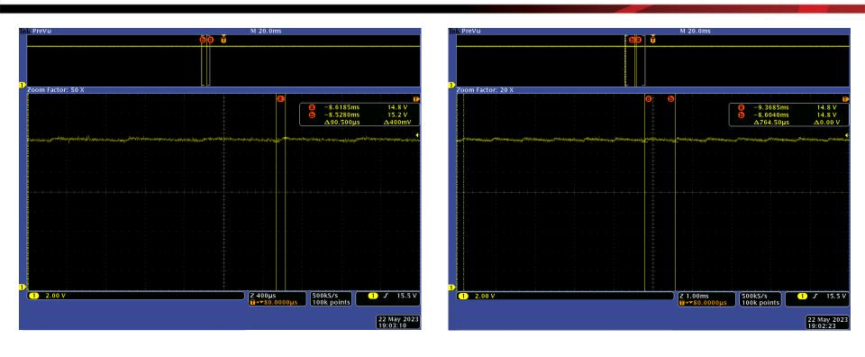
10% supply output measures 400 mV peak to peak, with a period of 1306 Hz
