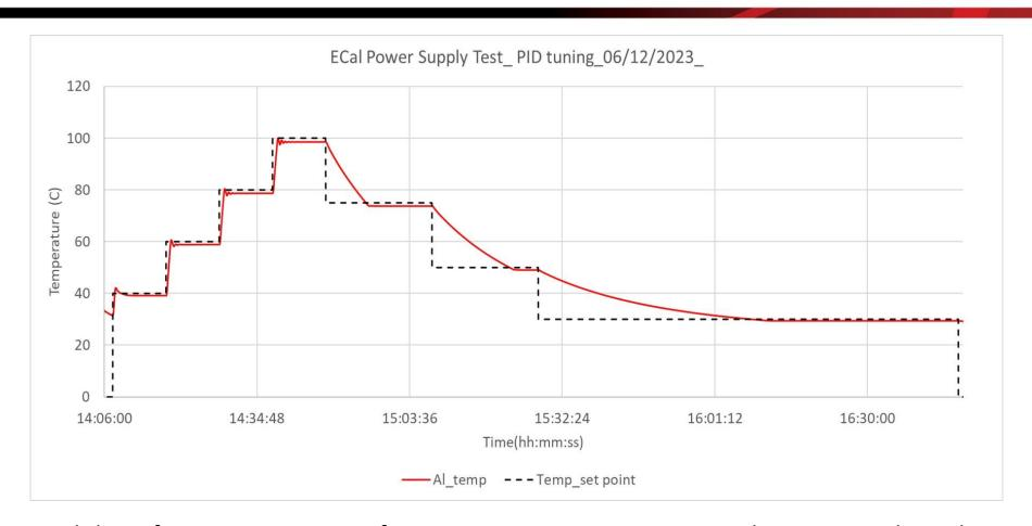
Tested the software over a range of temperature setpoints to ensure the PID controls work
