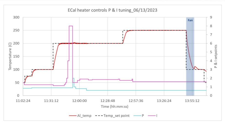
Fine tuning of the proportional and integral gains were done at temperatures up to 250°C
