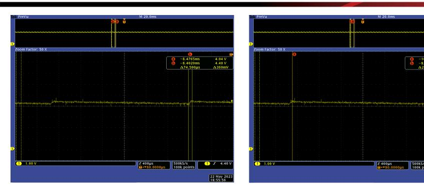
5% supply output measures 360 mV peak to peak, with a period of 395 Hz
