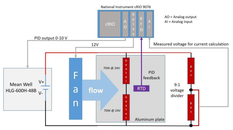
The test stand uses the Mean Well HLG-600H-48B (48 V, 600 W) supply to provide power to the two 70-W heaters. The PID controls software runs on the cRIO, which uses an RTD for feedback. Current and voltage are monitored by the cRIO as it reads ~10% of the output voltage using a voltage divider circuit. A fan is used to quickly lower the temperature, when needed.
