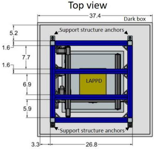
• Each vertical extrude has two gussets on the bottom (inside anchor gusset view obscured by the structure) that are used as anchor points to screw the structure to the dark box floor
