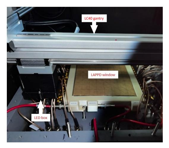
• The LED box was moved to the extreme front–left corner to ensure total window coverage in that direction
