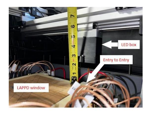
• The vertical distance measurement at Entry to Entry is ~2.5"
