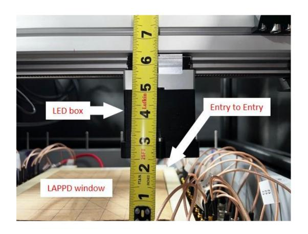
• The vertical distance measurement at Exit to Entry is ~2.6"
