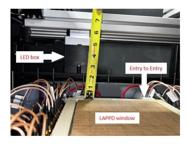
• The vertical distance measurement at Entry to Exit is ~2.5"
