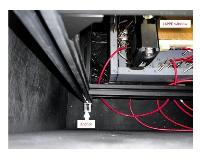
• During final installation, the anchor points will be fastened to the dark box with wood screws at all the vertical extrusions
