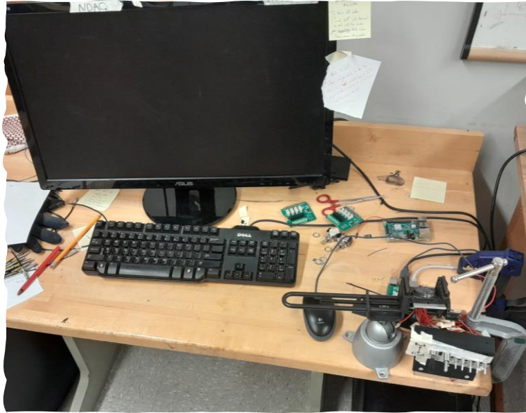
Fig. 6: LV test system with raspberry pi
