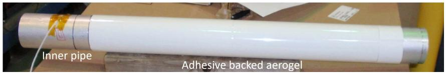
Aerogel insulation is added to the simulated beam pipe to prevent direct contact with the flow of air from the controls system
