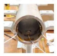
· Tested the RTDs using LabVIEW
