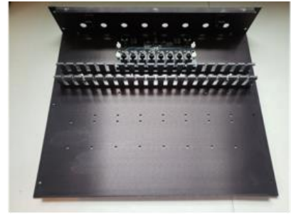
3. Cable management installed
