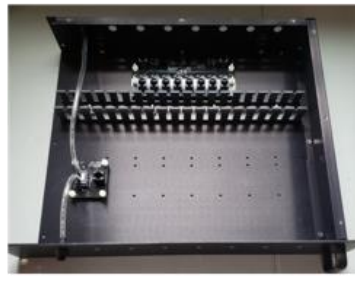
5. Side and front panel installed with gas connections and lines
