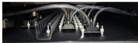
6. All channels installed with gas lines trimmed to length
