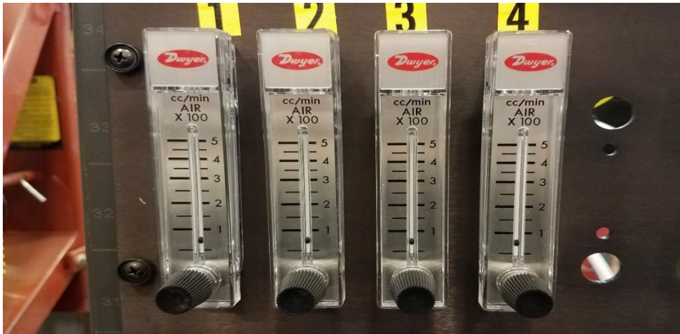
Figure 1. Flow set on the four standard flow rotameters
