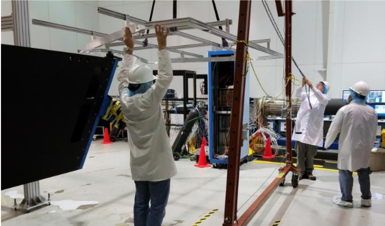
George Jacobs and Argonne Collaborators lifting assembled frame to place it on floor to glue Mylar/Tedlar sheet.
