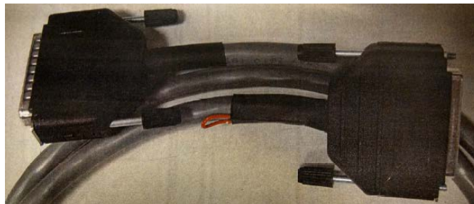
VME to patch panel cable.
