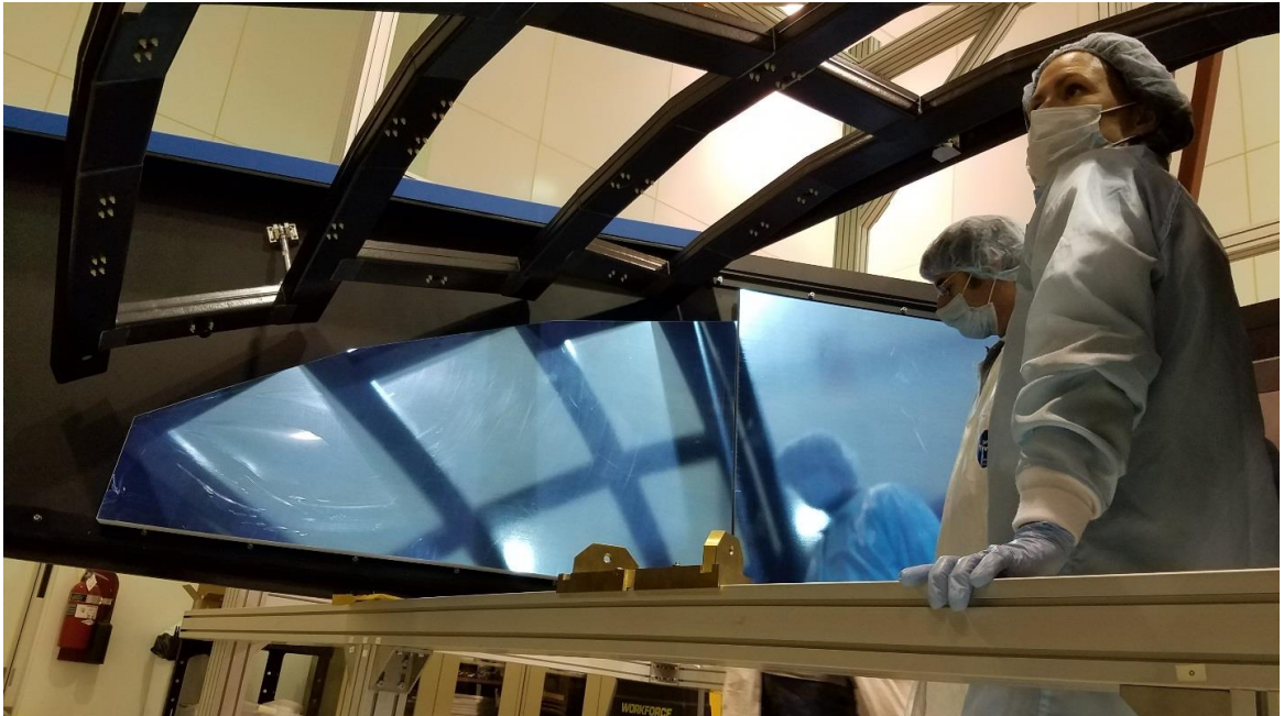
Mindy Leffel and Marco Mirazita with lateral mirrors inside assembly structure.
