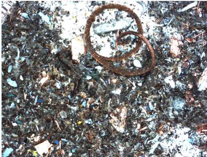
Debris found in MPS; long copper coil is ~6 mm in diameter.
