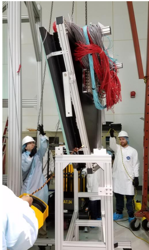
Tyler and Brian lifting E-panel with gantry crane.
