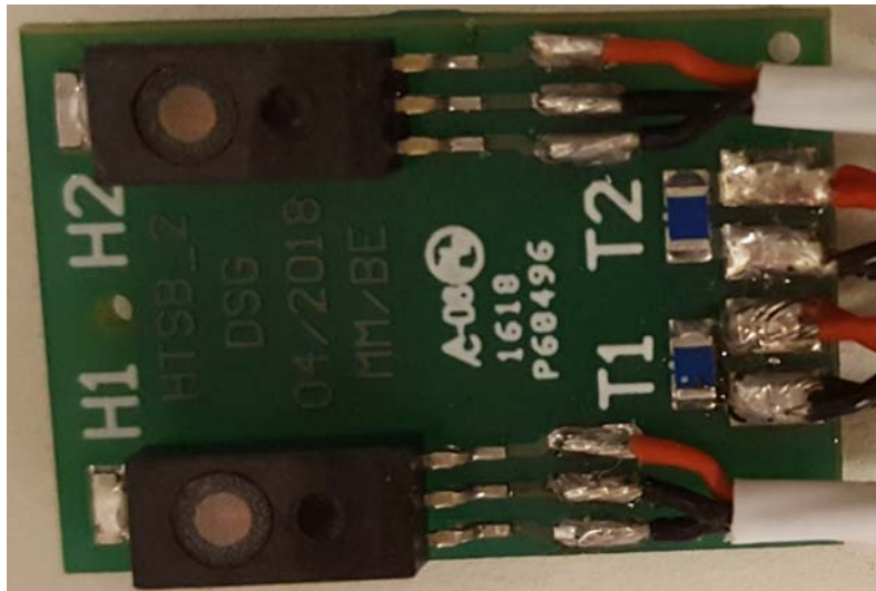
Humidity and temperature sensors at HTSB2 board
