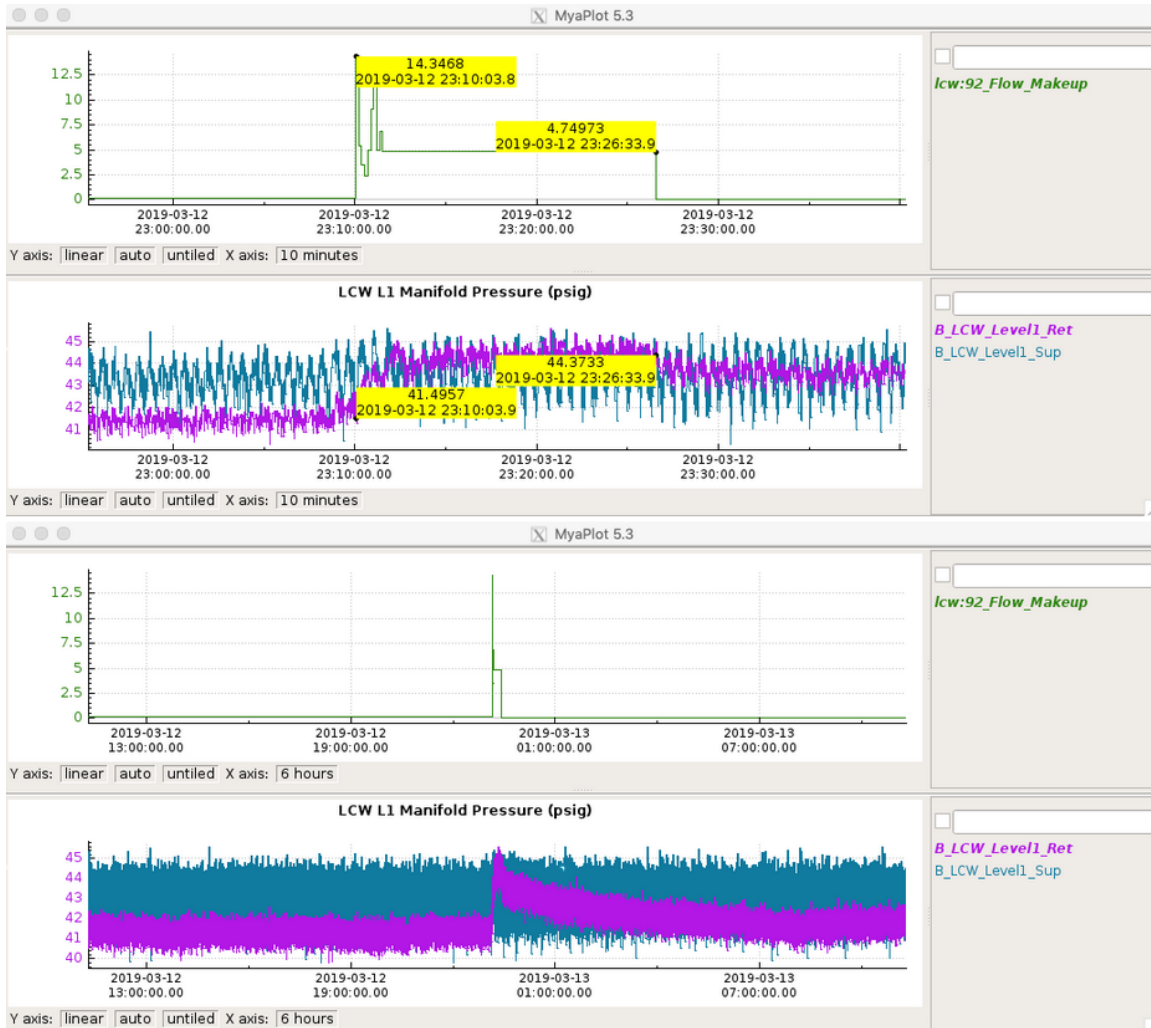
LCW return and supply values for makeup flow event, on 03-12-2019, after work done on tank.
