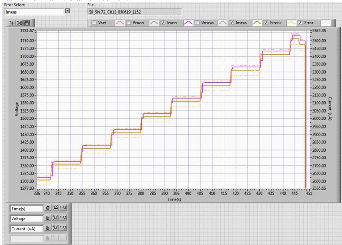
Figure 1. Module 72, channel 12 (~2625 \mu A to ~3550 \mu A). The magenta line is the current displayed from the CAEN, the solid orange line is the measured current. The dashed lines indicate the manufacturer's specification boundary.
