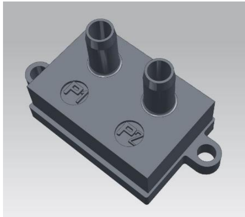
NX12 isometric view of flow sensor for GEM gas system
