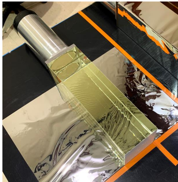
Glass block being wrapped with Mylar.
