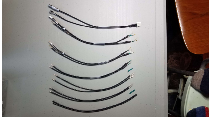
NPS HV diverter cables
