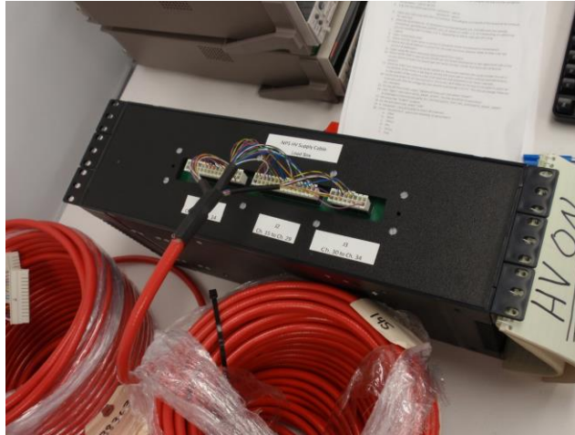
DSG designed load box for testing of HV supply cables
