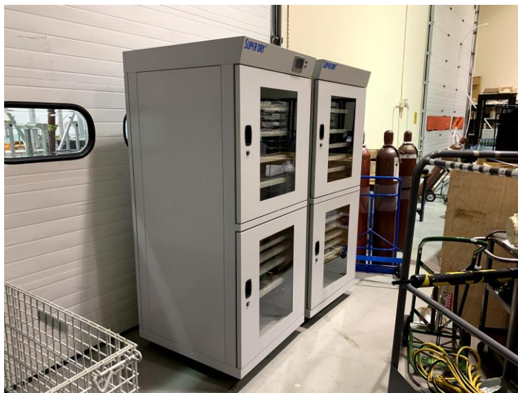
New dry cabinet in EEL 125 after installing wheels on to base of each section
