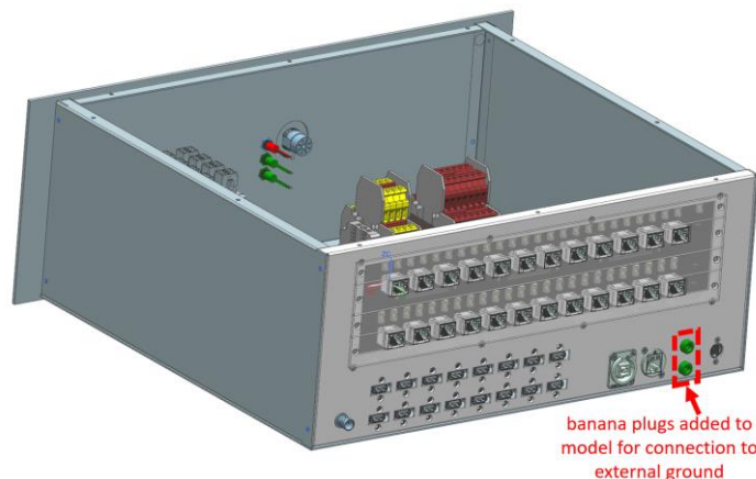
NX-12 model of hardware interlock chassis with banana plugs
