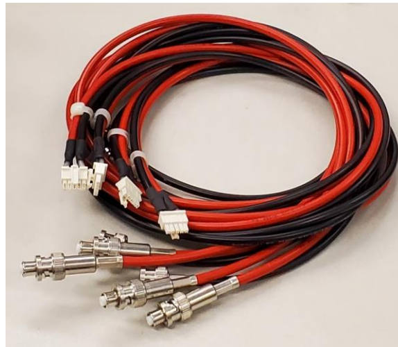
Terminated BNC-to-Samtec SHV cables
