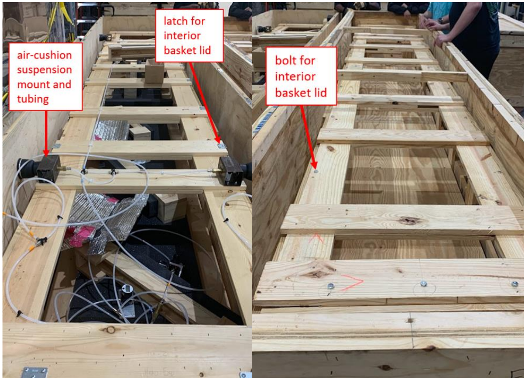
Left: interior of crate previously used to ship quartz bars, right: interior of new crates fabricated for quartz bar shipping.
