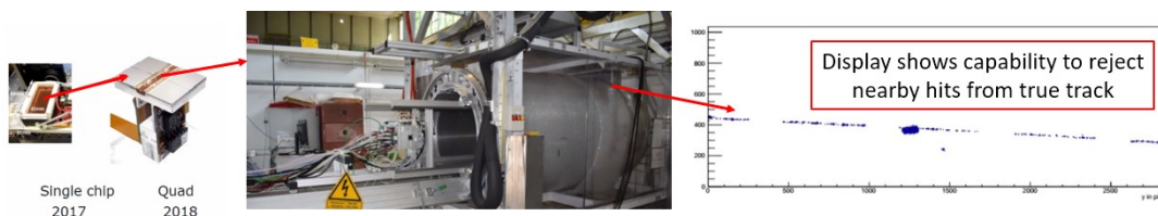
Figure 6: Building a set of chips into an array suitable for a test beam experiment.
