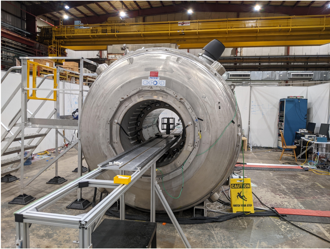
Figure 12: The magnetic solenoid at Argonne produces up to 5 Tesla for tracking resolution studies.
