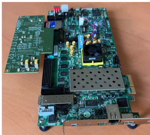
FIG. 5: Picture of a bare Carrier Board connected through FMC connector to a Xilinx ZC706
