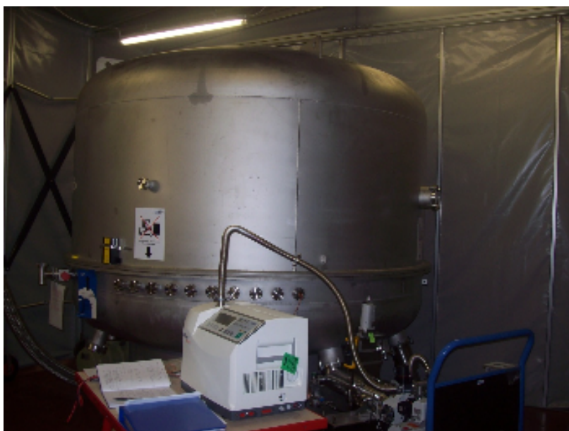
Fig.12 Test vacuum chamber and associated equipment
