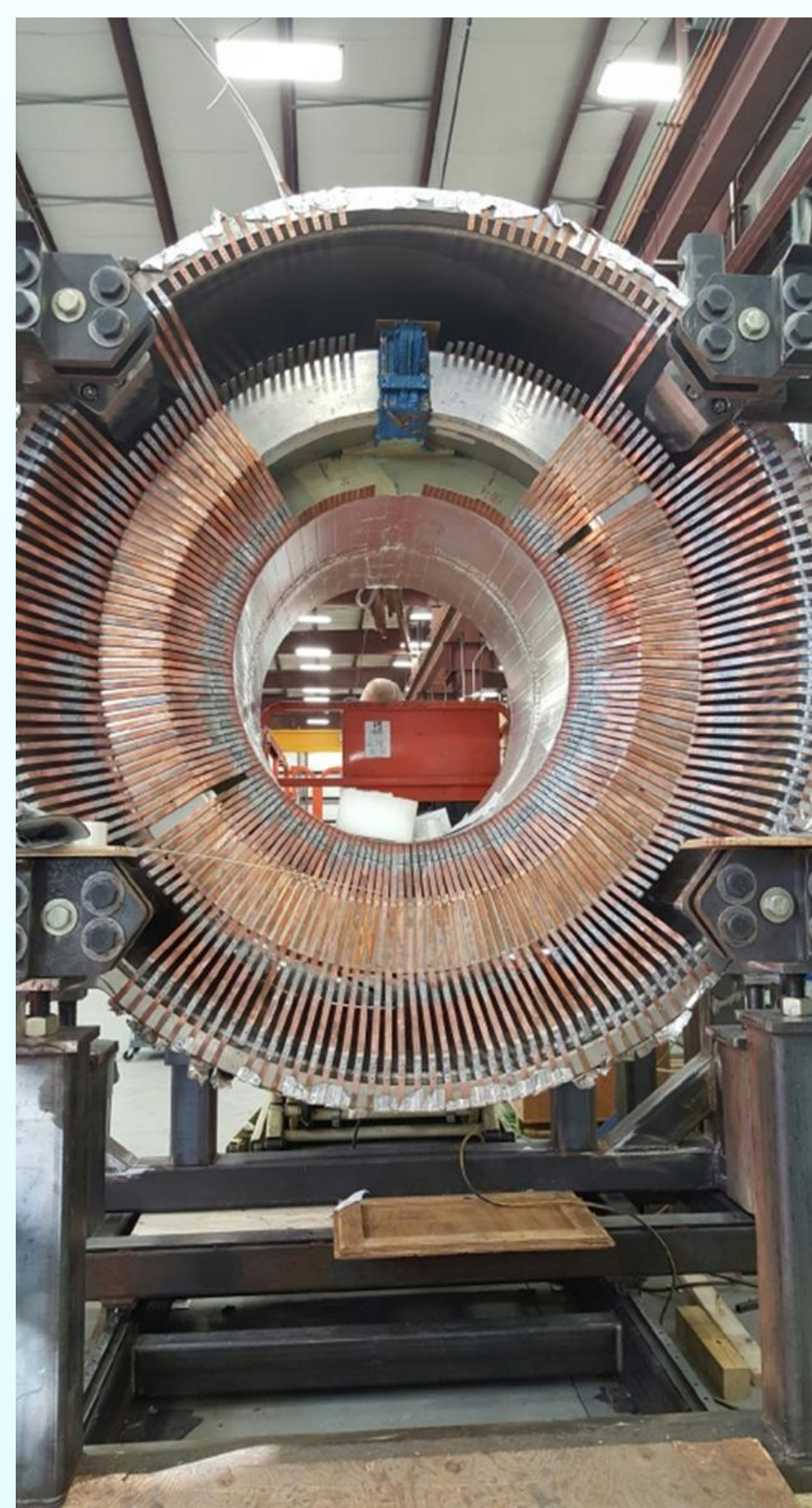
Installing the Copper cooling fingers which are used to cool the coils to liquid Helium temperatures
