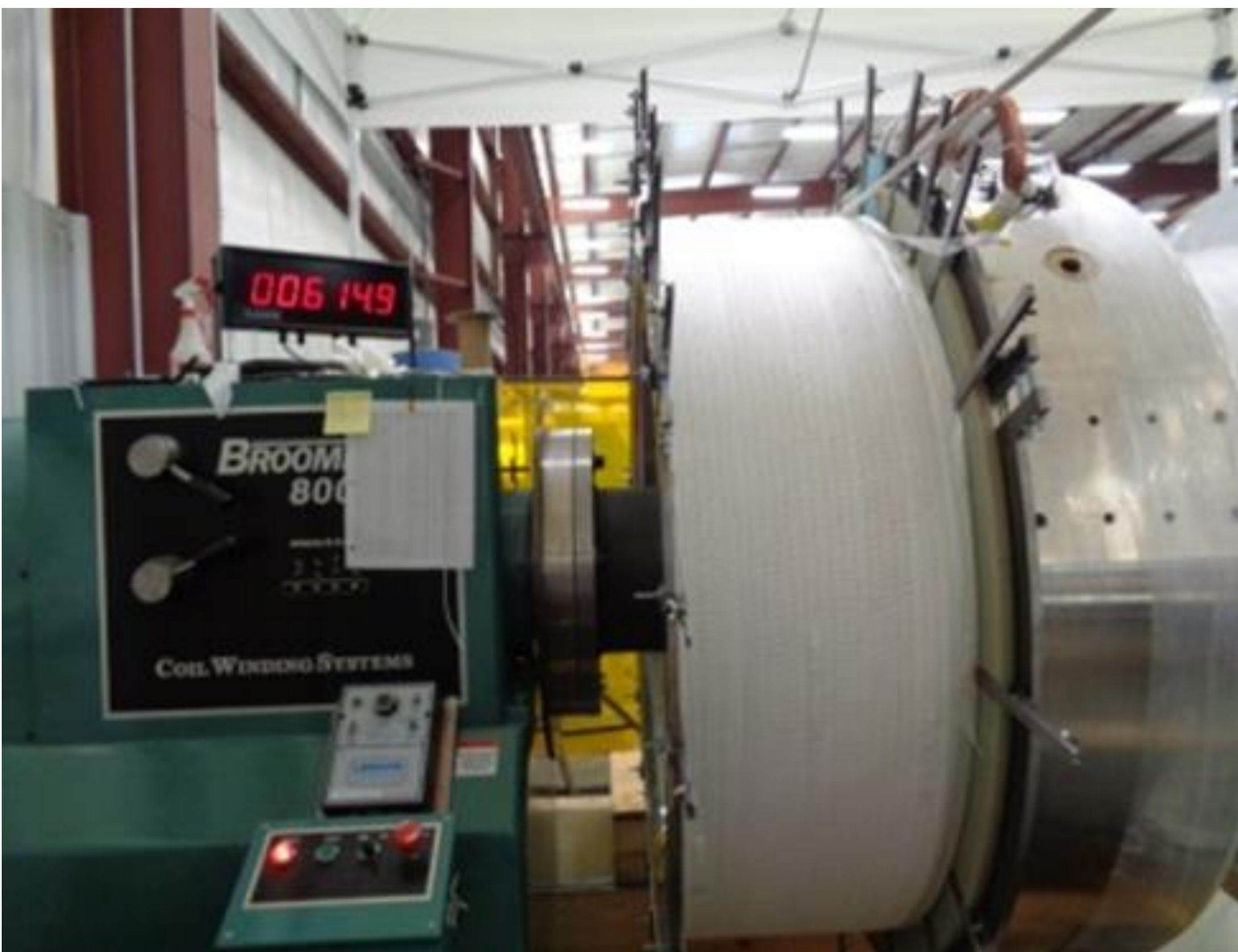
Superconducting coils being wound at Everson-Tesla Inc, Nazareth, PA
