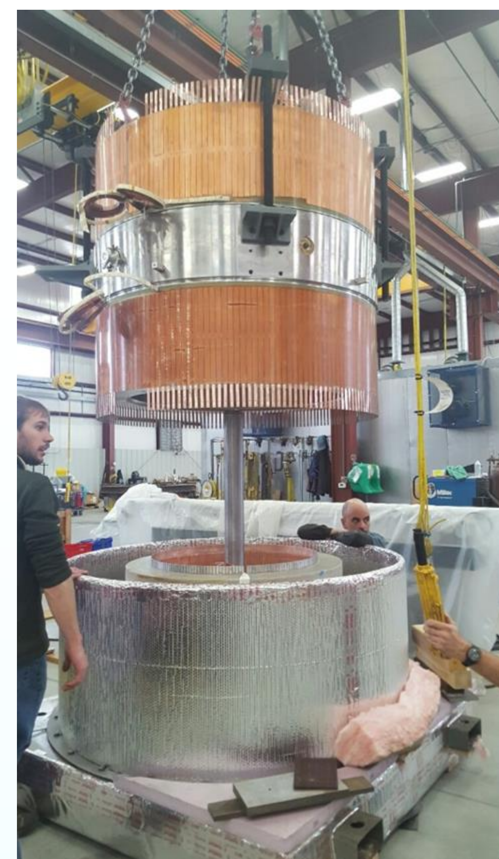
Superconducting coils being fitted together using liquid Nitrogen
