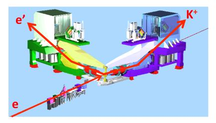
Two HRS spectrometers were used in time coincidence for the (e,e'K<sup>+</sup>) reaction: *L-HRS for scattered electrons (e')*
