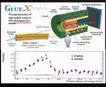
The GlueX experiment utilizes a linearly polarized photon beam constructed through coherent Bremsstrahlung radiation. The photons are tagged by the scattered electrons coming off of a diamond wafer. Once agged, the photons will then proceed to
