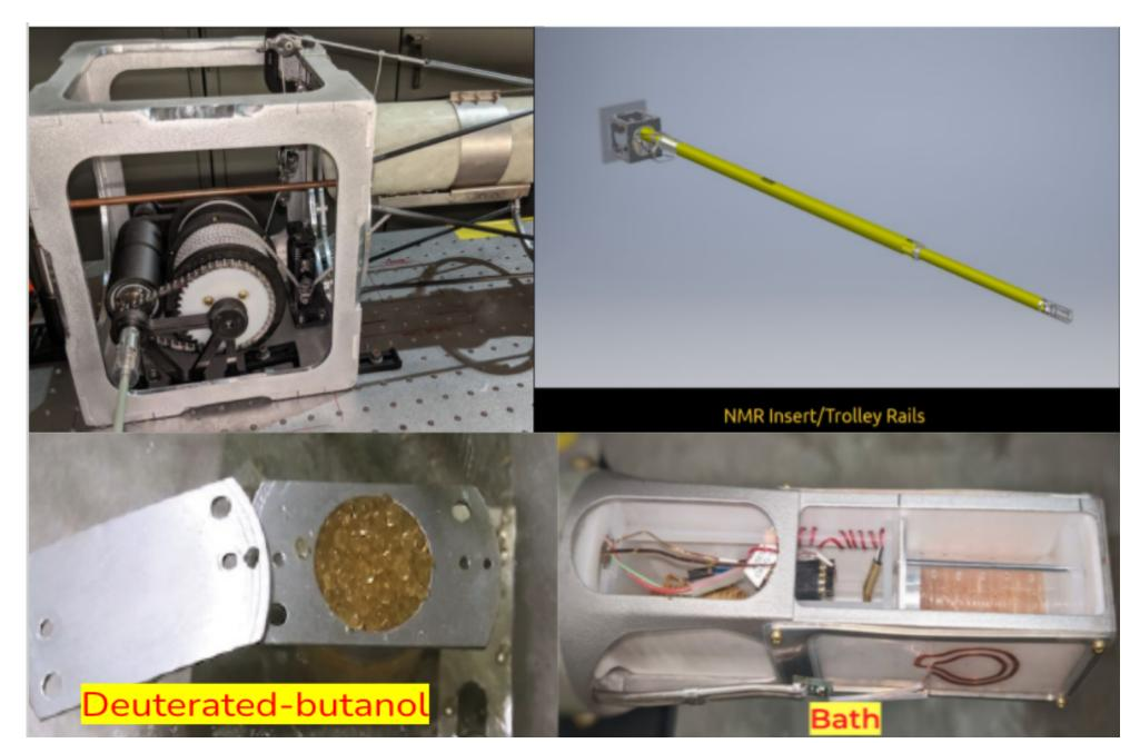
Dynamic Nuclear Polarization (DNP) is one of the most effective methods used to increase the nuclear spin polarization. Unpaired electrons polarize to over 99% in the magnetic field of 5 T at 1 K temperature at thermal equilibrium, while nuclei would have only 0.5% polarization. Microwave irradiation excites transitions that transfer the electron polarization to the nuclei, with over 80% achievable for protons.
