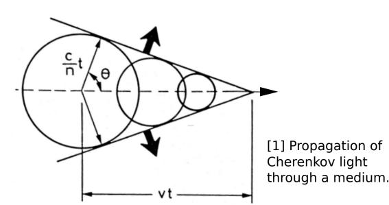
Electrons will have a greater velocity than a pion at the same momentum due to their smaller mass. A medium with a certain index of refraction can be chosen so that electrons will cherenkov and pions will not, up to certain momentum threshold. This momentum is often called the Pion Threshold.
