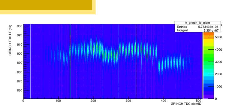
2D histogram of the LE for all the GRINCH PMTs, run 13460.
