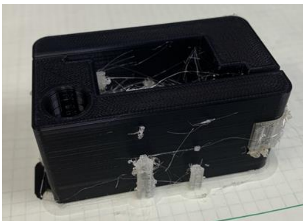
Printed horseshoe clamp. The white portions are polyvinyl alcohol supports that will be removed with water.
