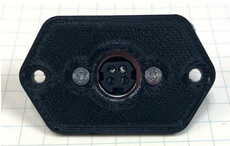
Front of adapter plate with locking, DC power port installed
