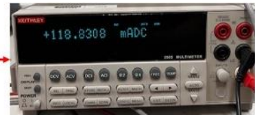
Max current flow through the 400 ohm resistor which is in parallel to the test load
