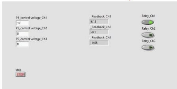
LabVIEW PSIC test software: Testing channel 1 at 100% current output
