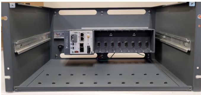
Inside view of partially fabricated cRIO chassis
