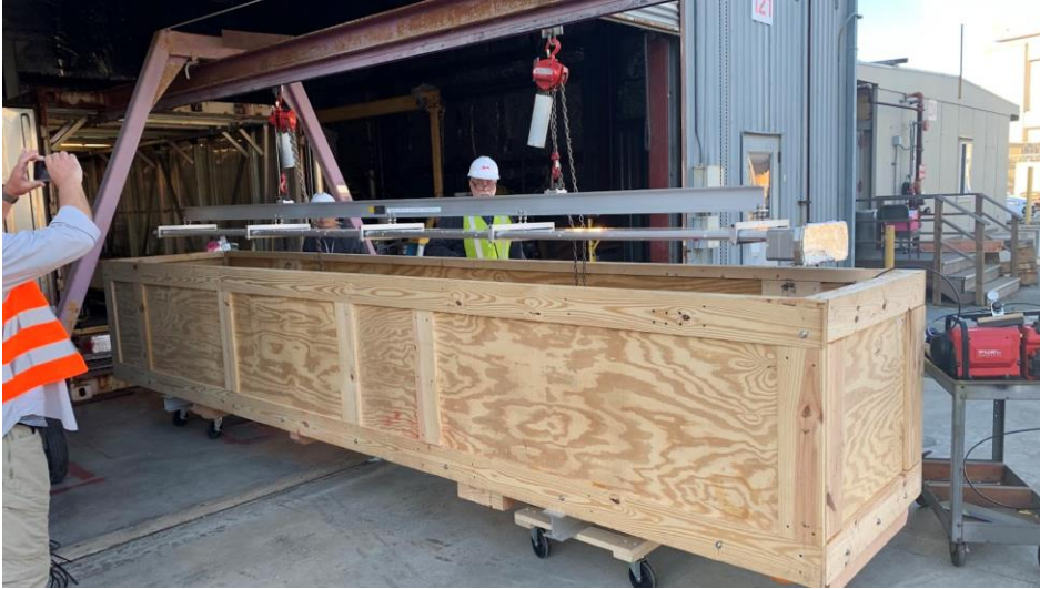
Barbox being loaded into a shipping crate at SLAC using their chain hoist and rail system
