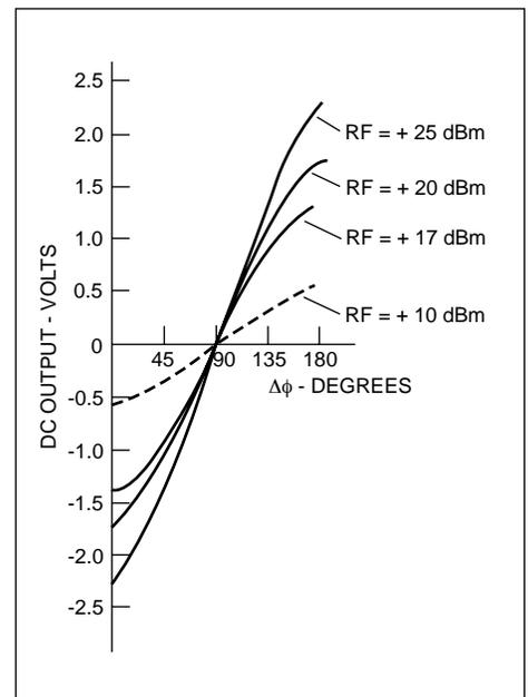
Figure 12. Increasing the RF level increases the maximum output voltage. (Data were taken at 30 MHz using an LO level of +27 dBm, and a load resistance of 50Ω.)
