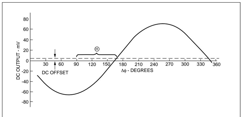
**Figure 10.** Data on dc output vs taken on a diode mixer demonstrates the effects of both dc offset and mixer-induced phase shift. The dashed line shows the effect of the dc offset. (Data were taken using a frequency of 1.5 GHz, an LO drive level of +6 dBm, an RF level of -9 dBm, and an IF load of 50.
