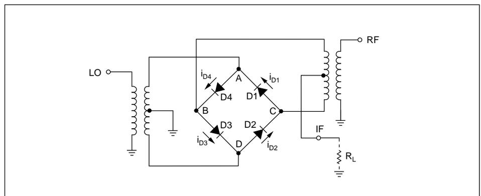
Figure 1. A typical double balanced four-diode ring mixer.
