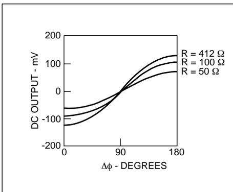
Figure 14. Increases in load resistance result in increased maximum output voltage. (Data were taken on a WJ-M6G mixer at a frequency of 1.85 GHz using an LO level of +6 dBm, and an RF level of -9 dBm. Increasing load from 412Ω to 825Ω did not appreciably change the results.
