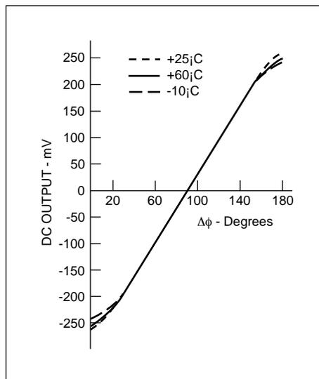
Figure 15. Effects of temperature variation on phase detector output. (Data using an LO level of 0 dBm, an RF level of 0 dBm, a load resistance of 1000Ω, and a frequency of 14,258 MHz.)
