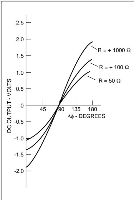
Figure 13. Increases in load resistance result in increased maximum output voltage. (Data were taken at a frequency of 30 MHz using an LO drive level of +27 dBm, and RF level of +17 dBm.)
