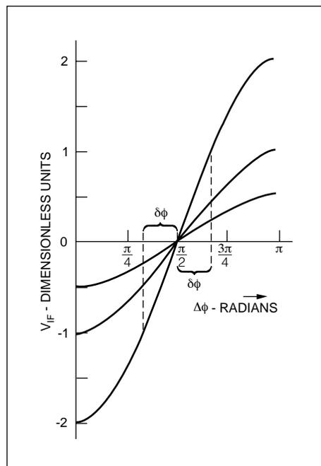
Figure 2. Typical phase detector response curve varies as cos (ΔΦ + π). Detector response is fairly linear over ΔΦ = π/2 + δΦ. Detector sensitivity increases as maximum V<sub>IF</sub> increases.
