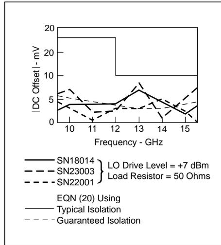
**Figure 5.** Magnitude of dc offset voltage as a function of frequency for three different WJ-M14A mixers. Also shown are results from equation 20 when typical and guaranteed isolation values for the M14A are used.
