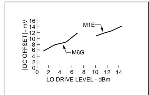
**Figure 6.** Magnitude of dc offset as a function of LO drive level of the WJ-M1E and M6G mixers. (Data on the M1E mixer were taken at a frequency of 210 MHz, with a load resistance of 1000Ω. Data on the M6G mixer were taken at a frequency of 1.5 GHz, with a load resistance of 50Ω.)
