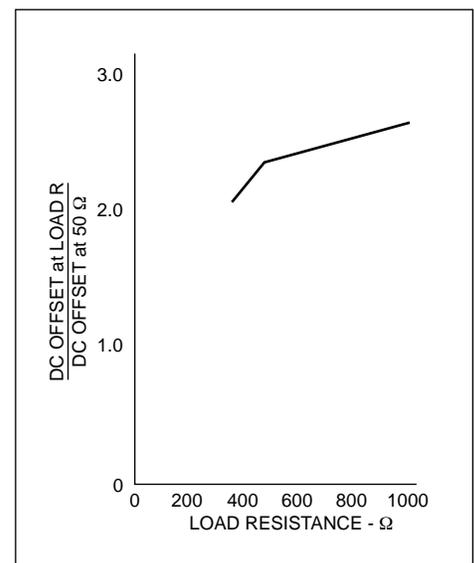
**Figure 7.** Increasing load resistance affects dc offset. (Data shown were taken using a mixer at a frequency of 210 MHz and an LO drive level of +14.6 dBm.)
