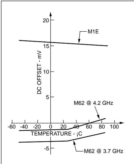
**Figure 8.** Changing temperature affects dc offset. (Data on the WJ-M1E mixer were taken at a frequency of 210 MHz, and LO drive level of +14.6 dBm, and a load resistance of 1000Ω. Data shown for 3 different units. These data were taken using an LO drive level of +6 dBm and a load resistance of 50Ω.)
