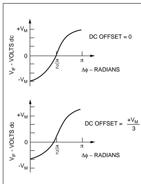
Figure 4. Non-zero dc offset voltage affects both the value of ΔΦ at which a null reading is obtained and the voltage measured for any given ΔΦ.
