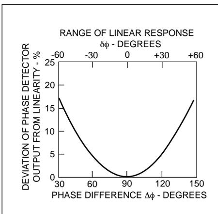
Figure 3. Phase detector output is a pseudo-linear function of phase difference.
