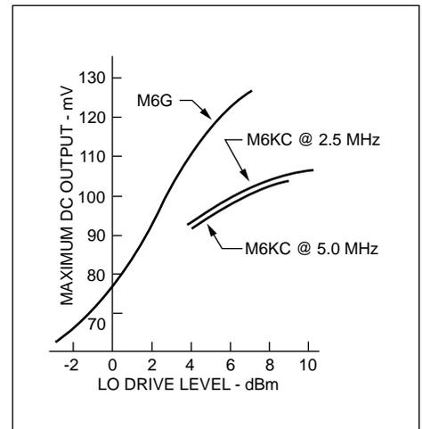
Figure 11. Maximum dc output voltage increases as LO drive level increases. (Data on the WJ-M6G were taken at 1.5 GHz using an RF level of -3 dBm, and a load resistance of 50Ω. Data on the WJ-M6KC were taken at frequencies of 2.5 and 5.0 MHz using an RF level of 0 dBm, and a load resistance of 50Ω.)
