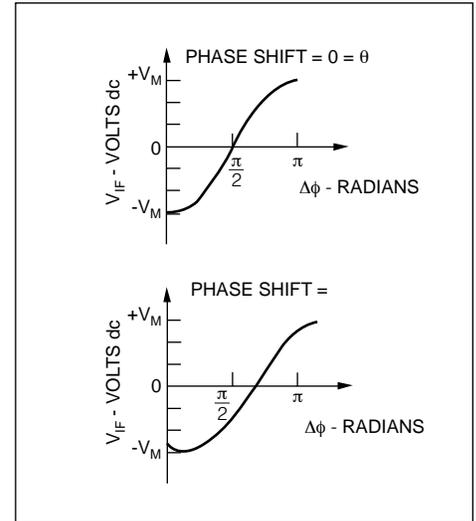
**Figure 9.** Mixer-induced phase shift  $\Theta$  affects the apparent relative phase at which a null reading is obtained. Minimum and maximum voltages are not affected, however.
