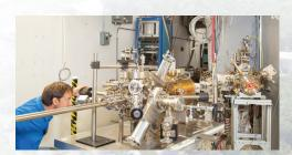
The injector produces electron beams for experiments.
